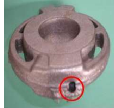
Fig 3. Cold shut defect
